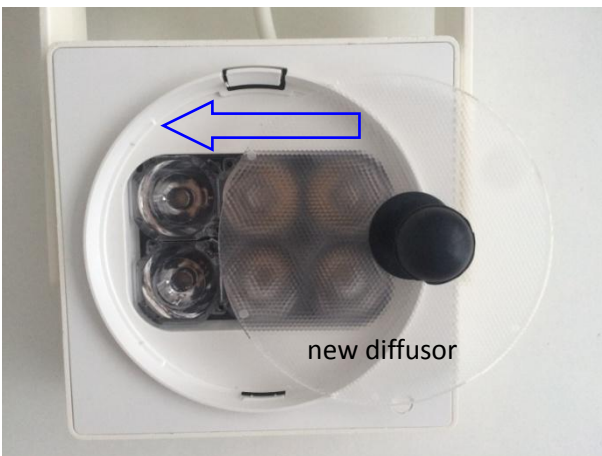
Step 4: Put in a new diffusor
