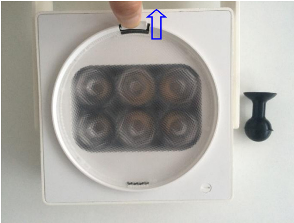
Step 4: Put in a new diffusor
